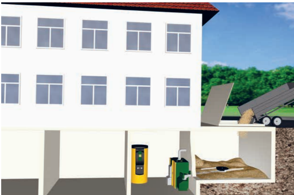
Heating system in the basement of a building KWB Multifire with stirrer and conveying channel; direct storage room filling from trailer
