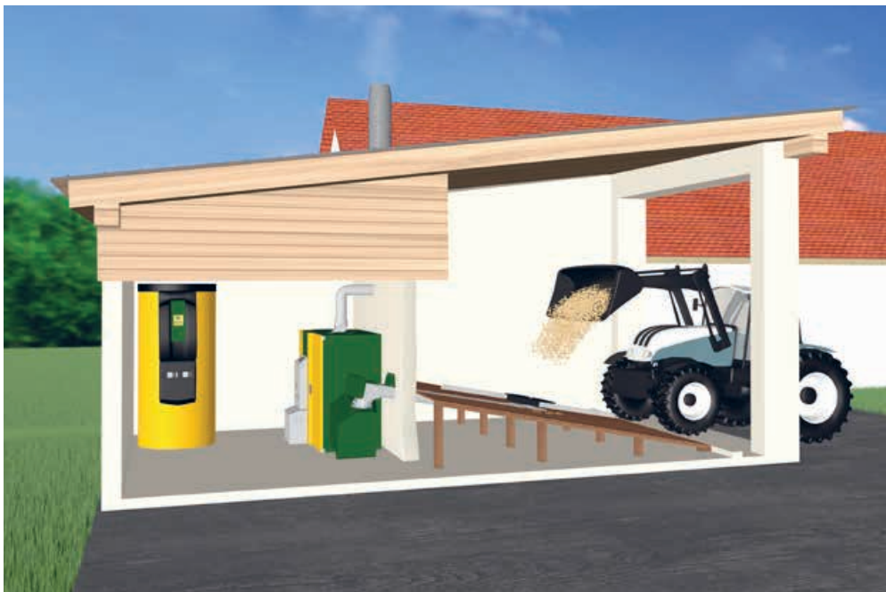
Heating system in adjoining building KWB Multifire with stirrer and conveying channel; direct storage room filling using tractor and front end loader
