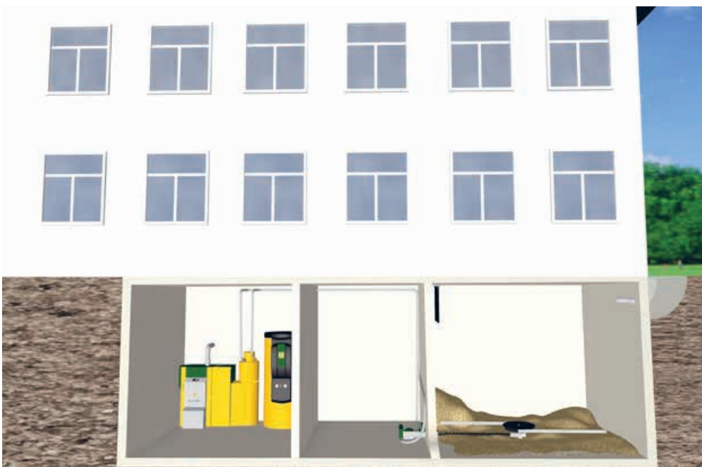
Heating system in the basement of a building KWB Pelletfire Plus with Pellet Stirrer Plus with suction conveyor
