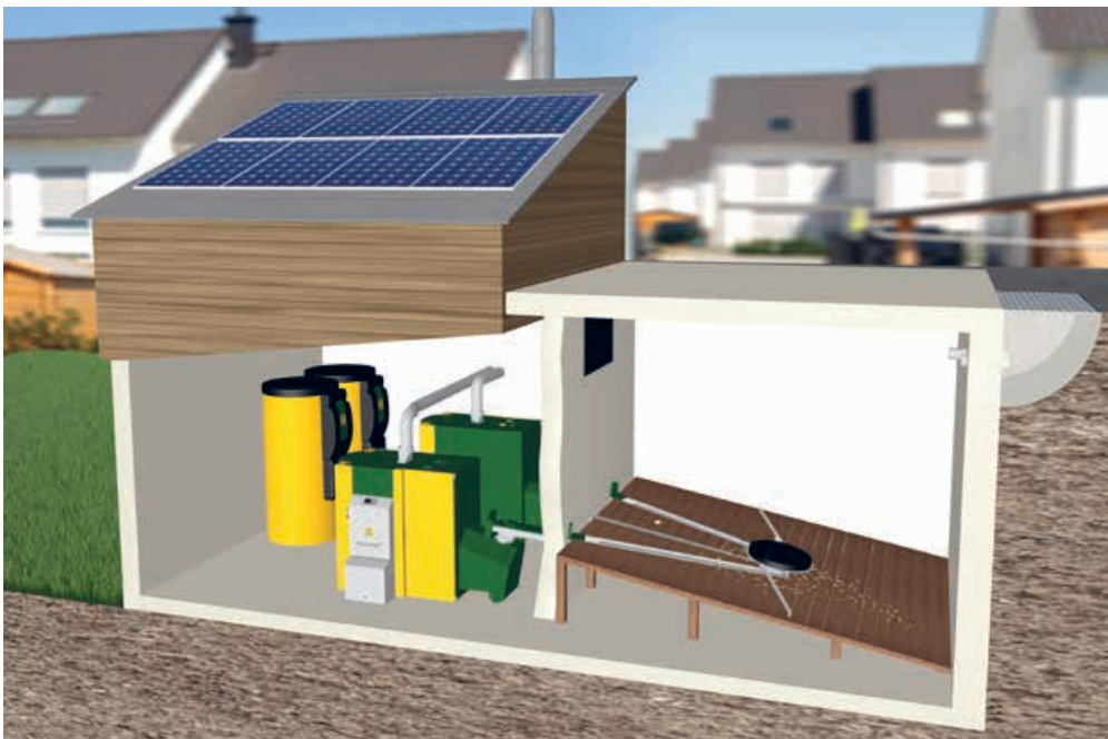
Heating system in separate boiler house KWB Pelletfire Plus twin boiler installation with common stirrer and two conveying channels;
